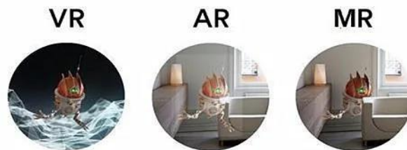
Figure 4 - (a) Digital environments that shut out the real world. (b) Digital content on top of your real world. (c) Digital content interacts with your real world. [10]
