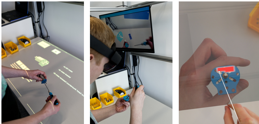
Fig. 5. The projection (left) and HMD system for assembly (center). The worker can take and annotate images for quality control in the QC application. in use.
