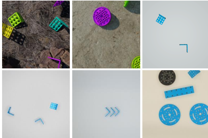
Fig. 4. Samples of the synth. training data in the first row (left and middle one generated by the data-generator, right one with Unity3D) and the real test data in the second row (left sparse, middle tight and right mul. class dataset)
