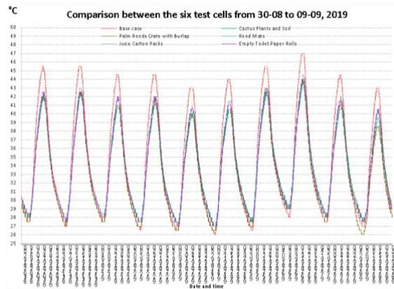
Figure 4: The monitoring results for the second 5 roof solutions compared to the base case and the outdoor temperature over summer.
