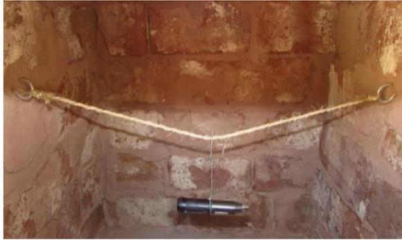
Figure 2. The logger hung in the middle of the test cell during monitoring.
