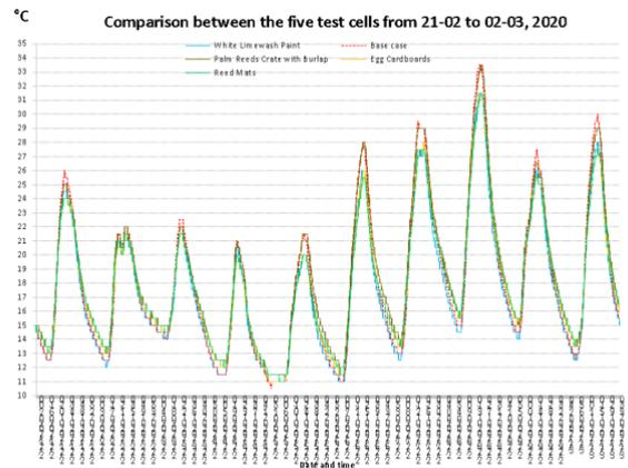
Figure 5: Monitoring results for the 4 best roof solutions compared to the base case and the outdoor temperature over winter.
