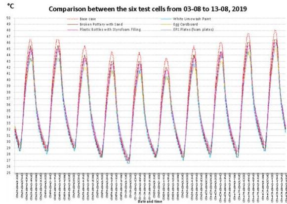
Figure 3: Monitoring results for the first 5 roof solutions compared to the base case and the outdoor temperature over summer.
