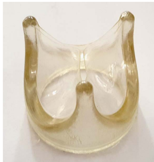
Figure 1: Final dip-casted 25-mm polyurethane valve.
