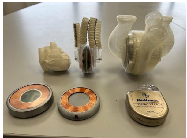
Figure 1: Size comparison Top from left: 5 years old heart model, resulted artificial heart, Bivacor TAH model; Bottom: Subcutaneous driver, smart battery, Medtronic Protecta XT CRT
