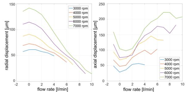
Figure 1: Radial (left) and axial (right) displacement for 3.5 mPa s and speeds from 3000 rpm to 7000 rpm.
