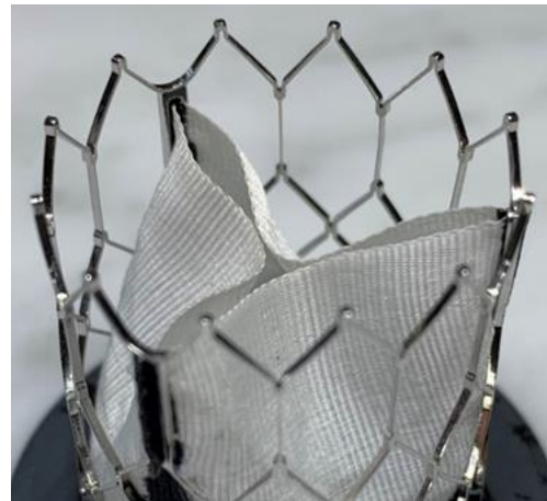
Figure 1: Textile heart valve scaffold tested with 200 million load cycles
